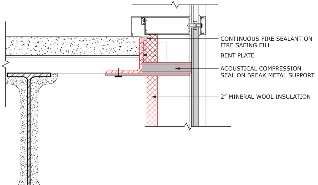
**Figure 14/15/16.05 – Field Conceptual Detail**
